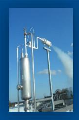
Both Phase Separators and Degassers automatically remove any excess gas phase out of the cryogenic system. Additionally, Phase Separators achieve a stable and predefined pressure at the application's outlet, intercepting pressure- and flow fluctuation from the supply.
